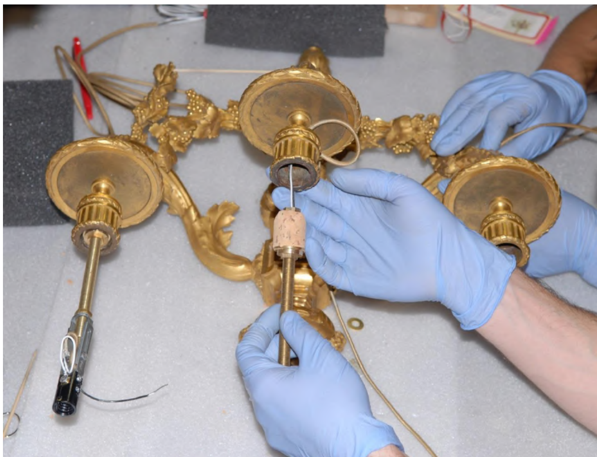
Fig. 7. Installation of electrical hardware and wiring on a three-light sconce. The Metropolitan Museum of Art, Gift of Mr. and Mrs. Charles Wrightsman, 1979 (1979.172.3) Photograph by the authors. © The Metropolitan Museum of Art
