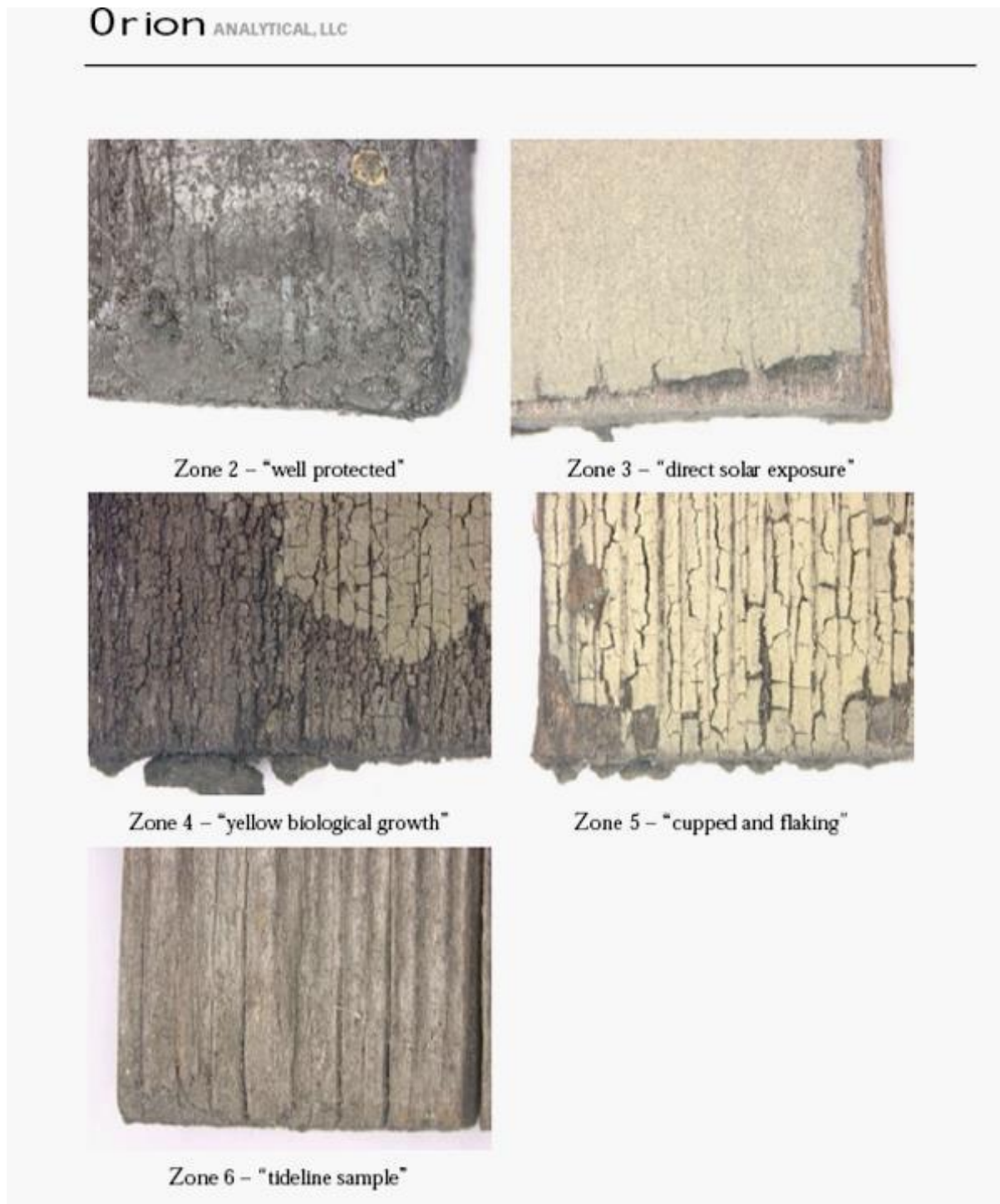
Fig. 4. Shake conditions before restoration. Courtesy Orion Analytical, LLC
